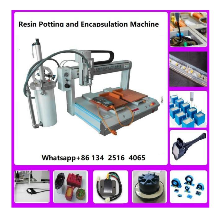
On the other hand, glue potting machines are designed to fill entire cavities or enclosures with adhesive material. They are typically used in applications where a part or assembly requires a high level of protection from environmental factors such as moisture, dust, or vibrations. Glue potting machines are used to apply a thick layer of adhesive to enclose and protect sensitive components such as circuit boards, sensors, or electronic assemblies
